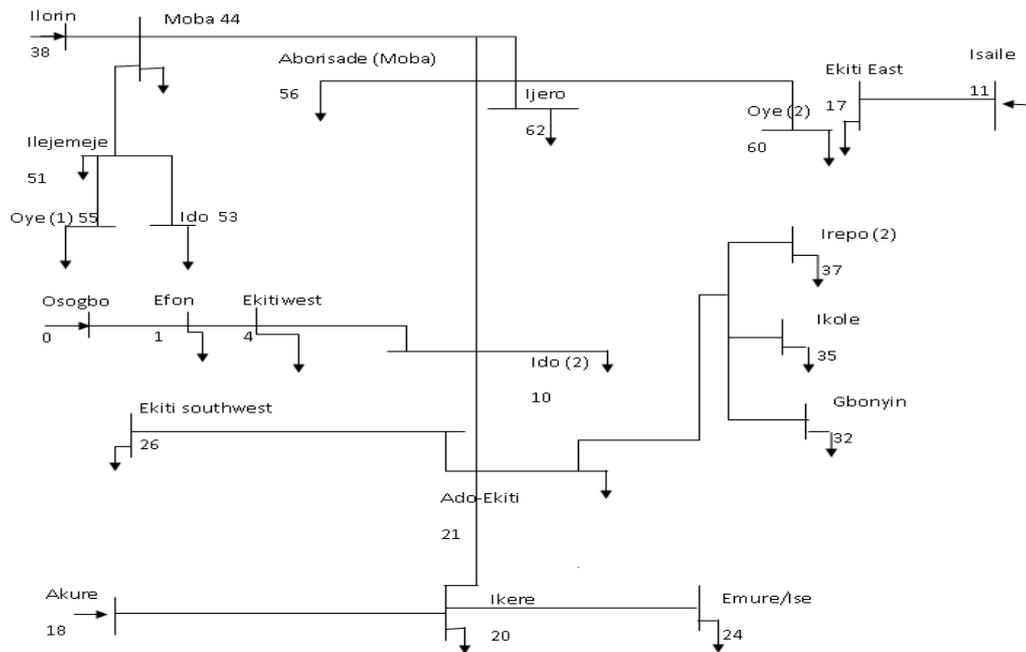
Figure 1: Simplified Ekiti 33kv Network
